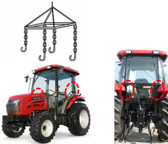
Fig.2-30 4 hangers to be lifted
